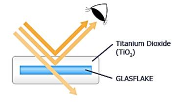
adjusting the coating thickness of the titanium dioxide, the optical path difference is varied and five colours of interference light are generated.
