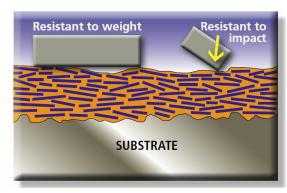
The glassflakes add tremendous strength to the coatings. The enhanced elongation and compression qualities provide superior resistance to the most severe abrasion and impact environments.
