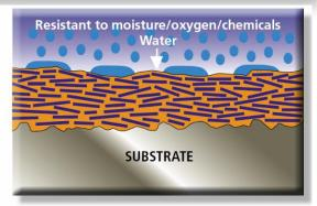
The glassflakes orientate as the film forms. The rigidity of the glassflakes combine with the strength of specially formulated resins creating impermeable protection barriers against abrasion and corrosion however hostile the environment.
